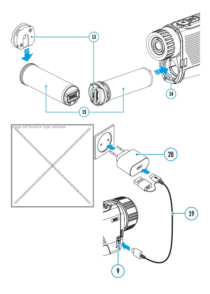
1. Install the APS 5 battery (15) in the battery compartment (14) of the
